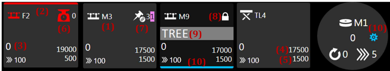
FIG. 19: DESCRIPTION OF THE MANUAL MODE TILE
